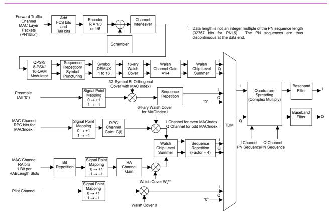
Figure 3-2 1xEV-DO Forward Block Diagram
