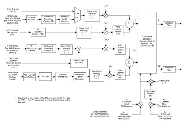
Figure 3-7 1xEV-DO Reverse – Block Diagram
