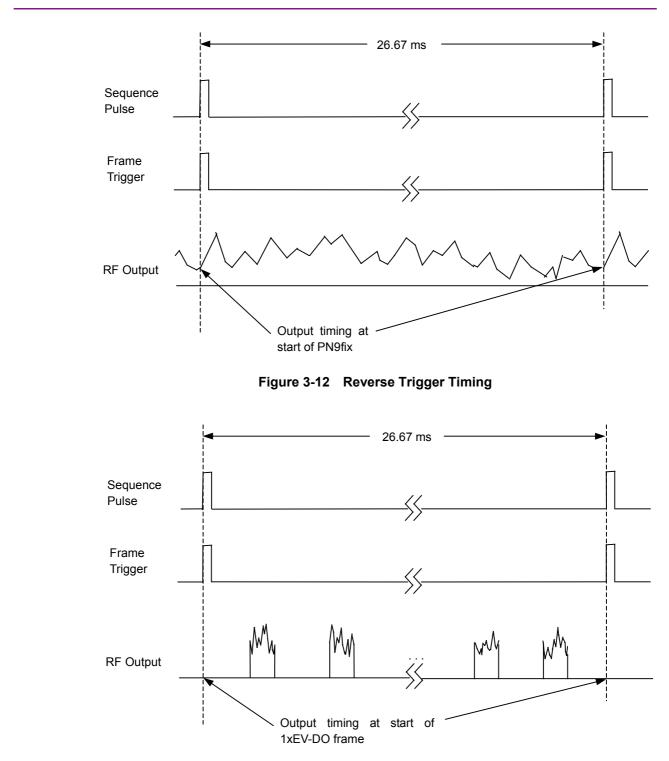
Figure 3-13 Trigger Timing for Forward Idle Slot
