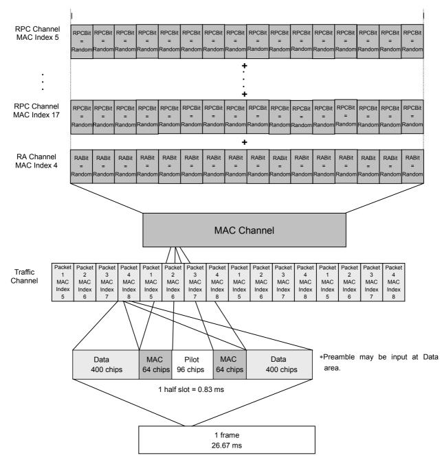
Figure 3-5 Multiplexing of each Channel
