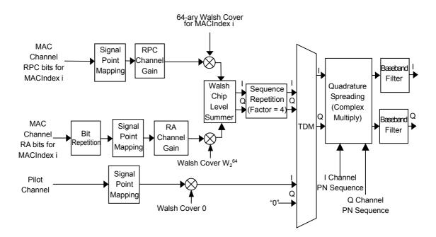
Figure 3-8 Forward Idle Slot – Block Diagram
