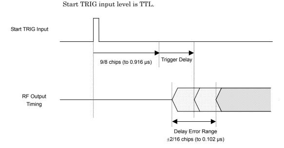
Figure 3-10 External Trigger Operation
