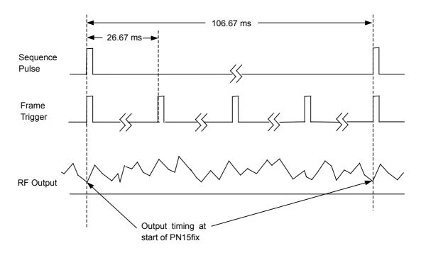
Figure 3-11 Trigger Timing for Forward (excluding Idle Slot)
